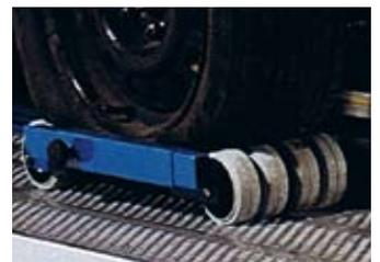
*The loading trolley allows you to load immobilized vehicles and can also be used as a vehicle safety stop (just flip it over).*
