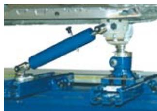
*Side support system locks parts in place when pulling, or holds them in place during welding operations.*
