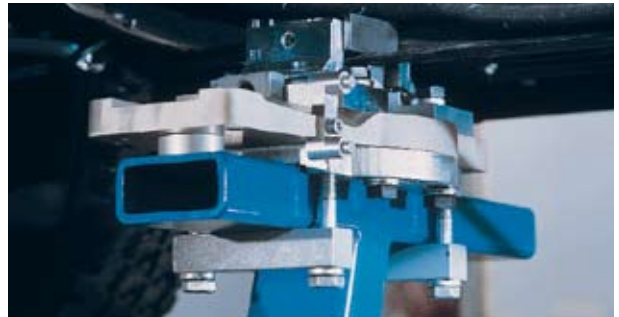
Vice-like clamp holds all frames effortlessly and precisely without collapsing the rails.
