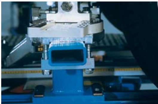
Clamps rotate to accommodate new angled frame designs.
